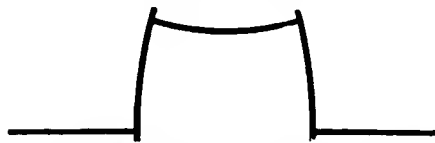
Fig. 1.—Illustrating effect of stresses on crank members.
